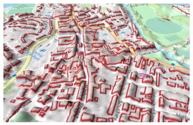
The algorithm uses this data to reconstruct roof shapes and to estimate which will receive sufficient sunlight throughout the year in order to be suitable for solar PV installation.
