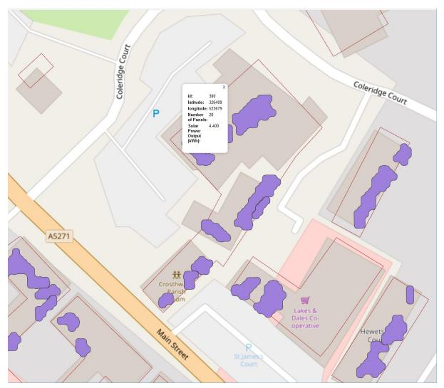
Roof areas are ordered so that the smallest id number "1" relates to the roof with the highest potential for solar power generation. So, we see that the roof area with biggest potential for solar PV is the Keswick Leisure Centre (there are also other potential roof spaces on this building).
